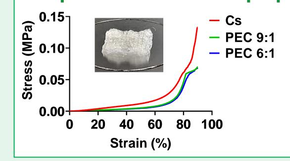
Cs samples were stiffer than PECs ones, as a consequence of the different fabrication parameters employed.
