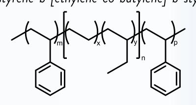
The polymeric film has been obtained by compression molding. SEBS has been employed with different amount of dispersed pyrene (1%, 2.5%, 5% and 10%).
