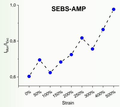
In SEBS-AMP, the deformation also increased the lifetime of monomeric emission (pyrene units are moved away from each other due to the external deformation and the aggregation becomes more difficult).
