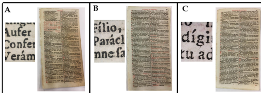
Figure 1. Images of pages and details from Breviarium romanum ad usum fratrum minorum treated with (A) water (pristine); (B) S_CNC; and (C) N_CNC.
