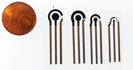
Figure 1. Screen-printed electrodes with 4, 3, 2 and 1 mm WE area, compared with 1 cent coin size.
