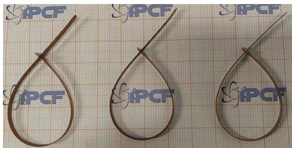
Figure 1. 3D-printed ties based on polymer/cutin blends
