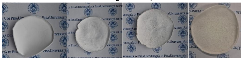
Figure 1. Images of the prepared composites: from left to right, neat PCL, 20%, 40% and 60 wt% rosemary fibers.
